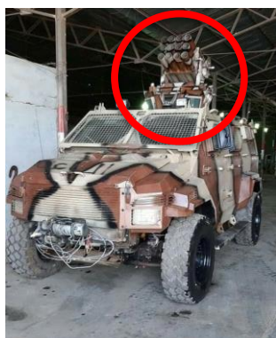
Figure B.36.3 KADDB Al Wahsh PPV modified with an 73mm SPG-9 recoilless gun fitted to 'snakehead' cupola c
