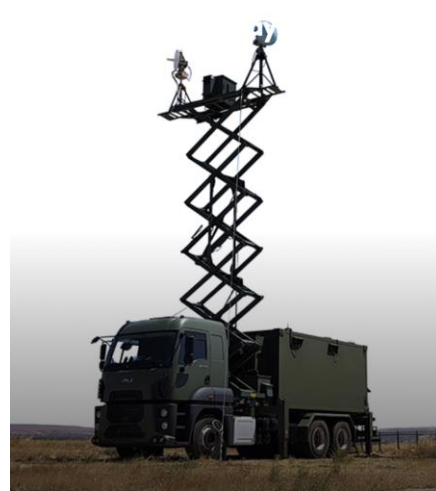
Figure 31.7 Ford 2533 trucks with C4 gantry on manufacturers' website
