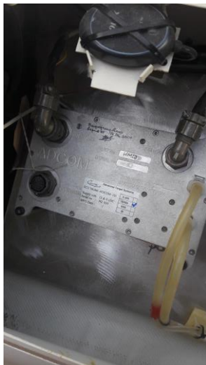
Image 51.20 ATS Fuel Control Unit Serial Number N2 039
